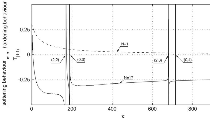
Fig. 11. Trend of non-linearity for mode (1,1). Single-mode approximation ( $N = 1$ , dashed line) and converged result ( $N = 17$ , solid line), are represented. The occurrence of 2:1 internal resonances with modes (2,2) ( $\kappa = 169.4$ ), (0,3) ( $\kappa = 187.9$ ), (2,3) ( $\kappa = 680.4$ ) and (0,4) ( $\kappa = 714.7$ ) are also shown.
