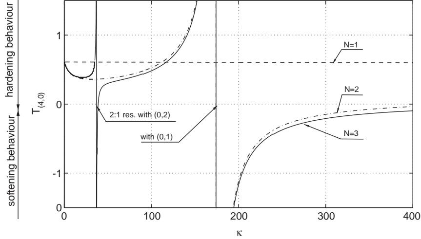
Fig. 6. Effect of the number of modes retained in the summations for the trend of non-linearity of mode (4,0). Dashed line ( $N = 1$ ): single-mode approximation. Dash-dotted line ( $N = 2$ ): (4,0) and (0,1). Solid line ( $N = 3$ ): (4,0); (0,1) and (0,2).
