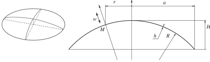
Fig. 1. Geometry of the shell: three-dimensional sketch and cross section.
