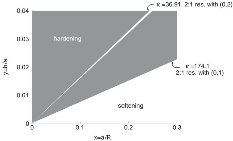
Fig. 5. Map of non-linear behaviour for mode (4,0).
