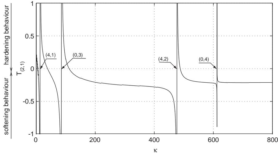
Fig. 12. Trend of non-linearity for mode (2,1), obtained with  $N = 18$  modes: (2,1), (4,0)–(4,4); and (0,1)–(0,6). 2:1 internal resonances with modes (4,1) ( $\kappa = 12.9$ ), (0,3) ( $\kappa = 85.5$ ), (4,2) ( $\kappa = 476.6$ ) and (0,4) ( $\kappa = 612.2$ ) are also shown.
