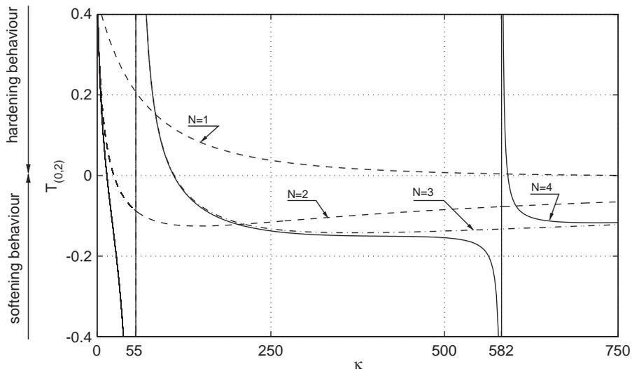
Fig. 10. Effect of the number of modes retained in the summations for the trend of non-linearity of mode (0,2). Dashed lines:  $N = 1$  (mode (0,2) only), and  $N = 2$ : (0, 1) + (0, 2). Dash-dotted line ( $N = 3$ ): (0,1) to (0,3). Solid line ( $N = 4$ ): (0,1) to (0,4).
