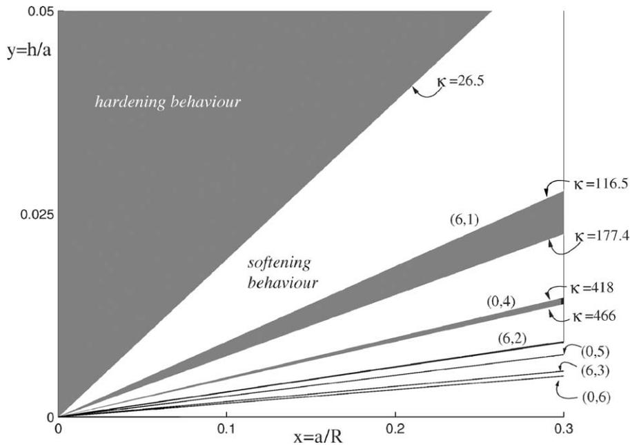
Fig. 13. Map of non-linearity for mode (3,1).  $N = 16$  modes have been retained for computation: (3,1), (6,0)–(6,3) and (0,1)–(0,6). Other 2:1 resonance occurs after (0,6), but are negligible and thus not represented.
