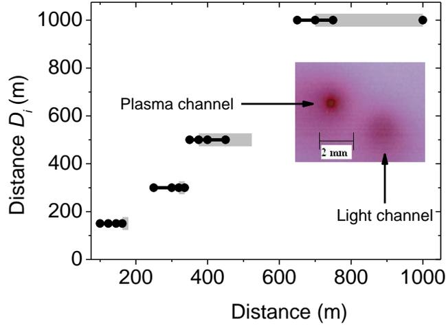
Fig. 2. Measurement of position of the plasma channels (black dot) and the position of the light channels (grey large line) for different distances  $D_i$ . Inset: impacts on a photographic paper showing a plasma channel and a light channel at 700 m for optimized parameters at 1 km.
