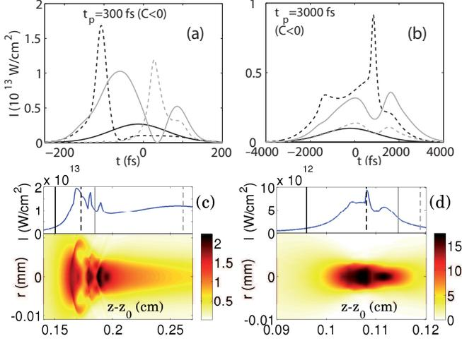
FIG. 6. Temporal intensity and plasma profiles at  $r = 0$  for several distances and input widths,  $t_p$ , of (a)  $-300$  fs and (b)  $-3$  ps. (c, d) Evolution across the nonlinear focus of (top) maximum of intensity and (bottom) fluence in  $\text{J}/\text{cm}^2$ . The color and style of the lines link the temporal profiles (a, b) with the distances marked by the vertical lines in (c, d), respectively.  $z_0 = 8.4$  (8.5) cm for left (right) column.
