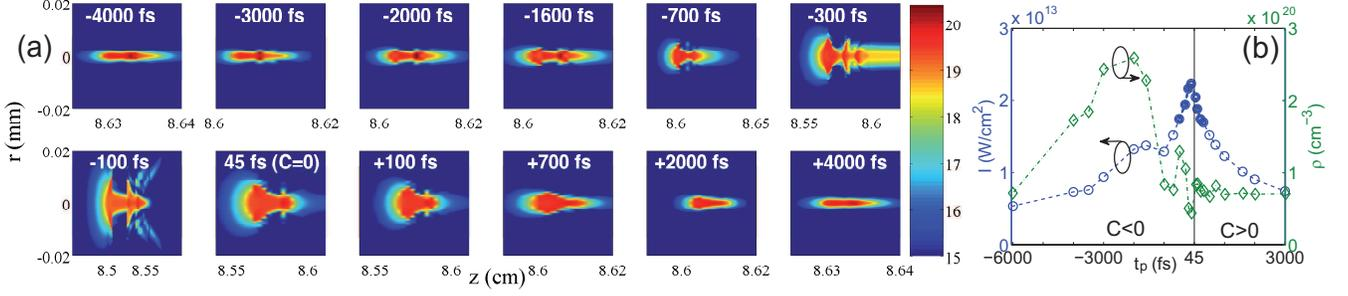
FIG. 5. (a) Plasma volumes around the focus for several initial pulse widths (marked by the labels). Densities are given by  $\rho(r, z) = 10^x \text{ cm}^{-3}$ , where the power  $x$  is given by the color bar. (b) absolute maxima of the electron density and intensity achieved in the focal volumes as a function of the chirped input pulse widths.
