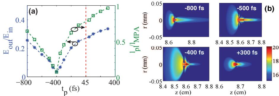
FIG. 7. (a) Transmission (left) and ratio of plasma absorption to MPA (right) as a function of the input pulse duration. Dashed vertical line marks the minimum pulse width ( $C = 0$ ). (b) Plasma volumes for several input pulse widths (see labels) and electron densities  $\rho = 10^x \text{ cm}^{-3}$ , where  $x$  is given by the color bar.
