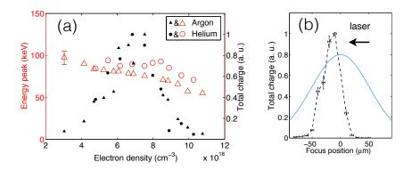
Figure 4. (a) Measured electron beam charge and peak energy over a range of plasma densities. The peak energy is computed from the weighted average energy over a spectral width at 90% of the maximum. (b) Electron charge measured by Lanex signal versus laser focus position relative to the center of the capillary nozzle. Z < 0 means laser is focused on the rear side of the nozzle. The blue line is the shape of a Gaussian density profile with a FWHM of  $120 \,\mu$ m.
