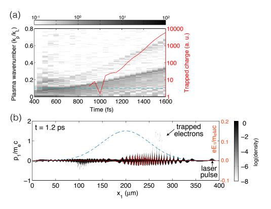
Figure 5. (a) The evolution of plasma wave number spectrum from the 3D PIC simulation. Solid curve (red) is the total charge of the trapped electrons defined as those with  $p_e/m_ec > 0.2$  which corresponds to a kinetic energy of about 10 keV. (b) The electron momentum phase-space  $(x_1, p_1)$  at t = 1.2 ps. Dashed curve (blue) is a lineout of the Gaussian density profile. Solid curve (red) is the normalized on-axis longitudinal electric field  $E_1$ . The laser travels from left to right.
