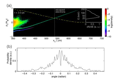
Figure 7. (a) The electron phase space  $(x_1, p_1)$  at t = 3.0 ps. Dashed curve (yellow) is the plot of the additive inverse of the longitudinal electric potential expressed in  $sgn(\phi)\sqrt{(|\phi|/m_ec^2+1)^2-1}$ . The energy distribution of the escaped electrons defined as those with  $E + \phi > 0$  is shown in the inset. (b) Angular distribution of the escaped electrons in the simulation.
