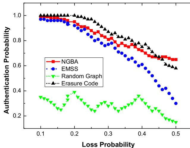
Fig. 8. Authentication probabilities at different loss probabilities. (The overheads is 30 bytes per packet)
