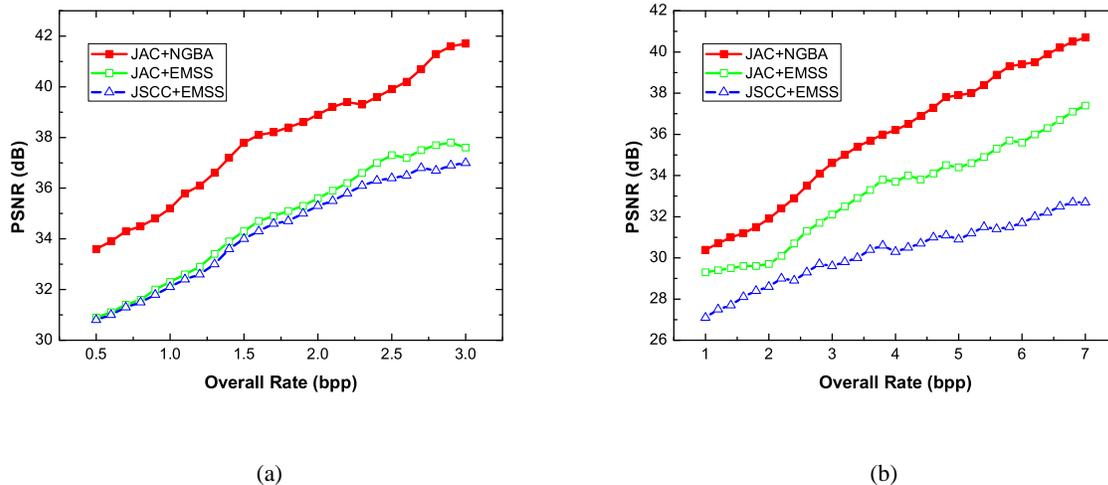
Fig. 9. End-to-end rate-distortion curves. (a) packet loss rate is 5% ( $r_a = 0.4$  for JSCC+EMSS). (b) packet loss rate is 15% ( $r_a = 0.25$  for JSCC+EMSS).
