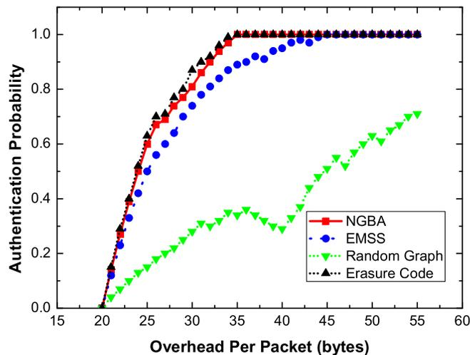
Fig. 7. Authentication probabilities at different overheads. (Packet loss probability is fixed at 30%)
