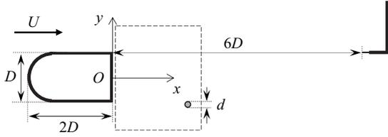
FIG. 1. Sketch of the experimental layout at the spanwise center section ( $D=25$  mm,  $d=3$  mm). The dashed rectangle represents the area explored by the control cylinder. The hot wire probe is depicted in the right hand side of the image.
